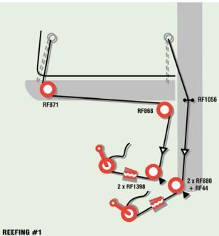
Basic 2 line reefing system. (2 lines per reef - single reef only shown) Suitable for yachts to 13m (43ft).
